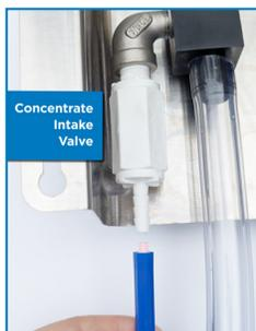
4. Drop the other end (weighted end) of the suction tube into the concentrate container.
